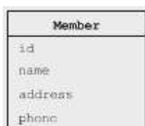
Figure 2.3 UML diagram for the class Member
